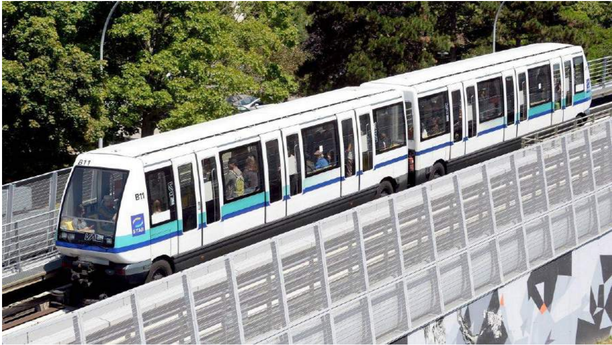
Fig 2.7 The Driverless, Rubber-Tyred, Rennes Metro
