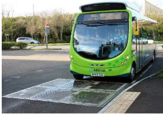
Fig 3.2 A wireless charging system (120kW units) has been in daily use in Milton Keynes since 2014
