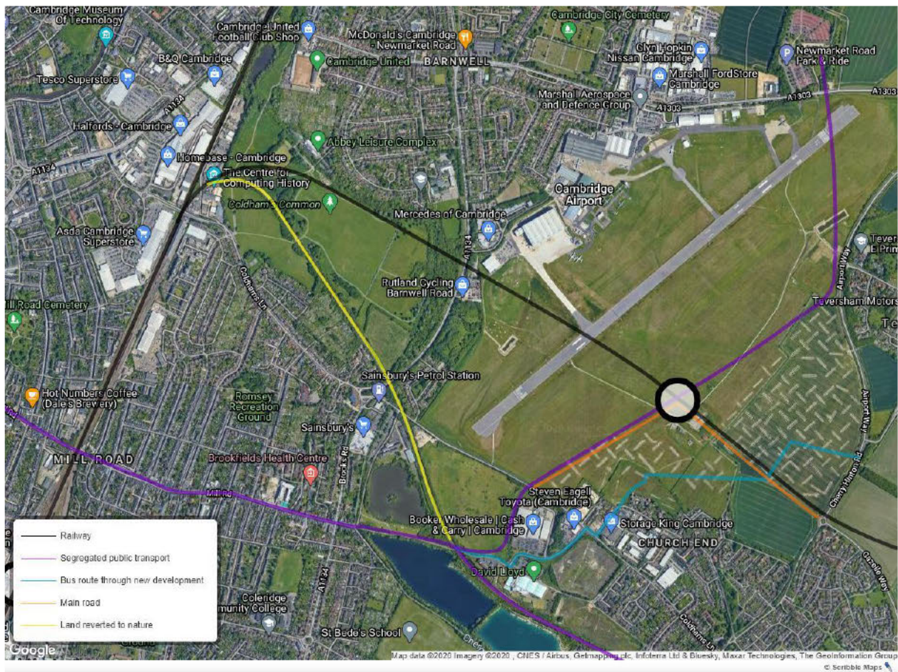
Figure 7: Zoomed-in detail of suggested railway realignment and public transport routes in east Cambridge
