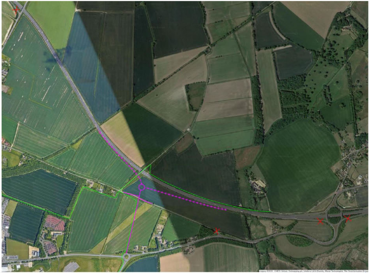
Figure 8: New A14 westbound junction to replace westbound slips on A14 Junctions 34 and 35 (pink = road, green = cycleway, red cross = access closed)
